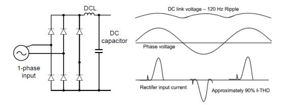
Figure-2 Typical Single-Phase Configuration
