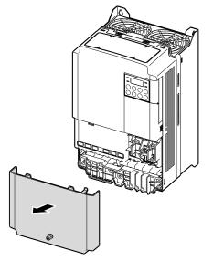
2 Push and hold the levers on both sides of the cable guide (1) and then remove the cable guide by pulling it directly away from the front of the inverter (2). In some models where the cable guide is secured by a bolt, remove the bolt first.
