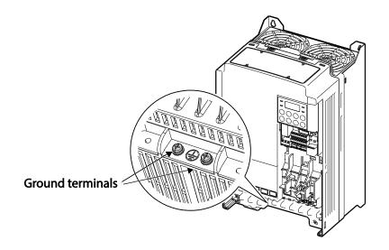
2 Connect the other ends of the ground cables to the supply earth (ground) terminal.
