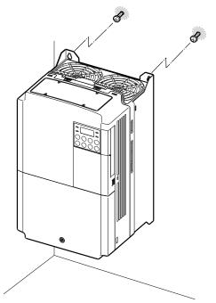
3 Mount the inverter on the wall or inside a panel using the two upper bolts, and then fully tighten the mounting bolts. Ensure that the inverter is placed flat on the mounting surface, and that the installation surface can securely support the weight of the inverter.
