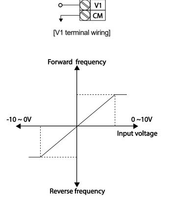
[Bipolar input voltage and output frequency]
