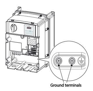
2 Connect the other ends of the ground cables to the supply earth (ground) terminal.
