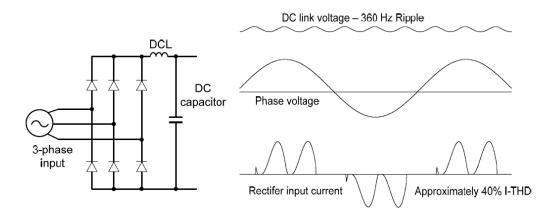
Figure-1 Typical Three-Phase Configuration
