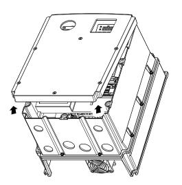
2 Set the bushing to every wiring hole before installing to power and I/O board terminals. Use the bushing that is NEMA 4X (IP66) or more.
