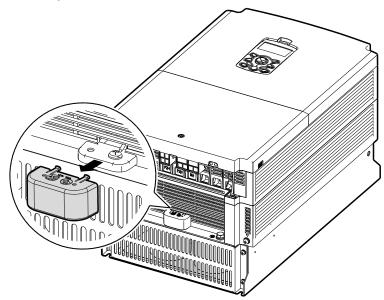
2 Remove the EMC ground cable from the right terminal (EMC filter-ON / factory default), and connect it to the left terminal (EMC filter-OFF / for power sources with asymmetrical grounding).
