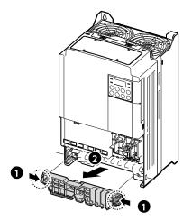
**3** Push and hold the tab on the right side of the control terminal cover. Then remove the cover by lifting it from the bottom and moving it away from the front of the inverter.
