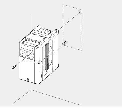
0.4kW (Single Phase) and 0.4-0.8kW (3-phase) inverters have only two mounting brackets.
