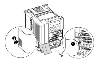
3 Connect the cables to the power terminals and the control terminals. For cable specifications, refer to <u>1.5 Cable Selection</u> on page <u>12</u>.
