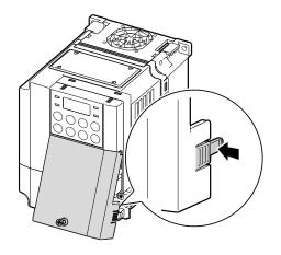
2 Remove the bolt that secures the front cover (left side) (①). Push and hold the latch on the left side of the cover. Then remove the cover by lifting it from the bottom and moving it away from the front of the inverter (②).
