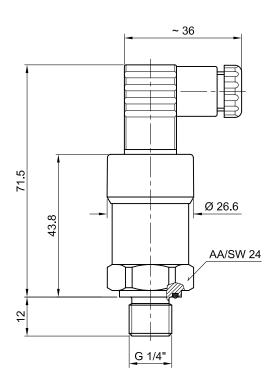
Thread connections can be either G1/4" or G1/2" upon request. (EN-837) Standard sealings are made up of Viton (0...60 bar) and NBR (>60 bar) The minimum permissible medium and ambient temperature for those is -30 °C
