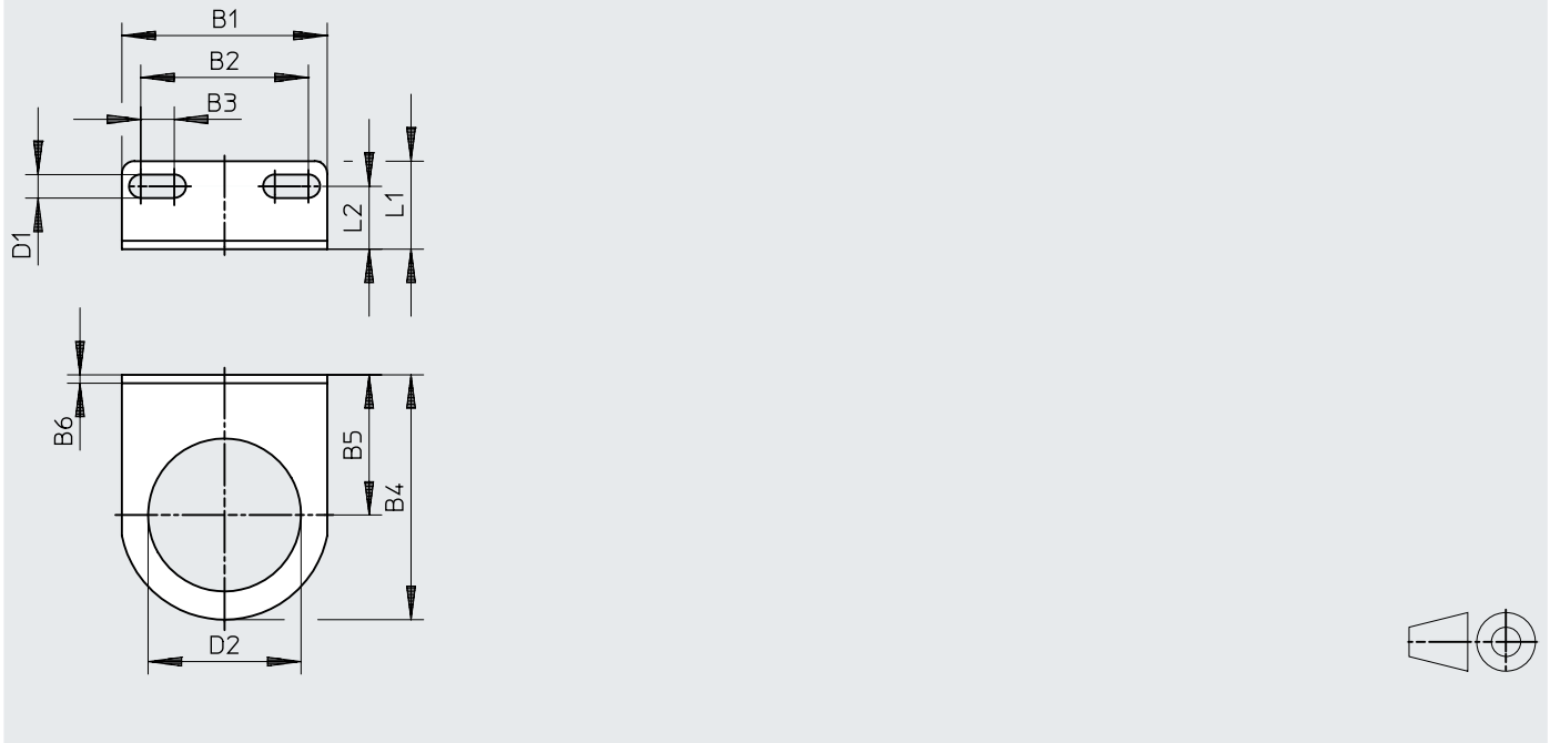
Dimensions – Mounting bracket HR
